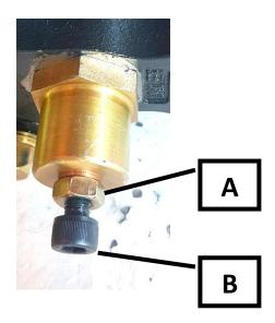
1) Unscrew the nut A, carefully keeping the hex screw B
